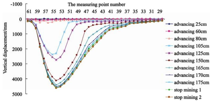
Fig.4 Changing curves of vertical displacement of the 2nd measuring line
