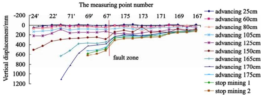
Fig.6 Changing curves of vertical displacement of the 4th measuring line
