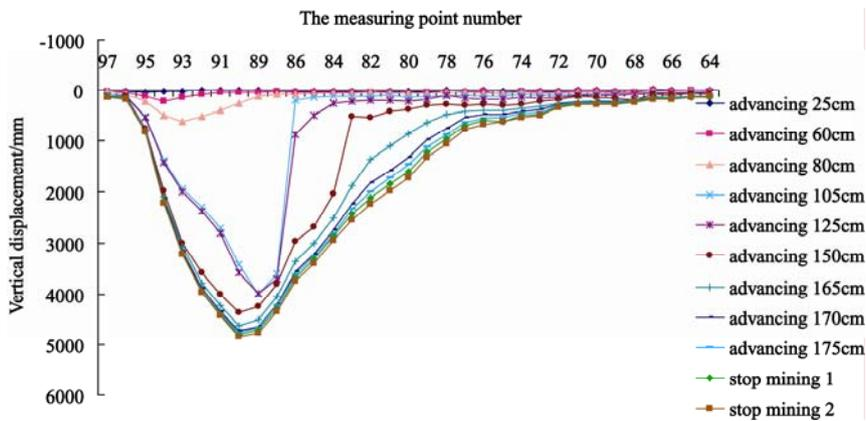
Fig.5 Changing curves of vertical displacement of the 3rd measuring line
