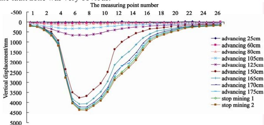
Fig.3 Changing curves of vertical displacement of the 1st measuring line
