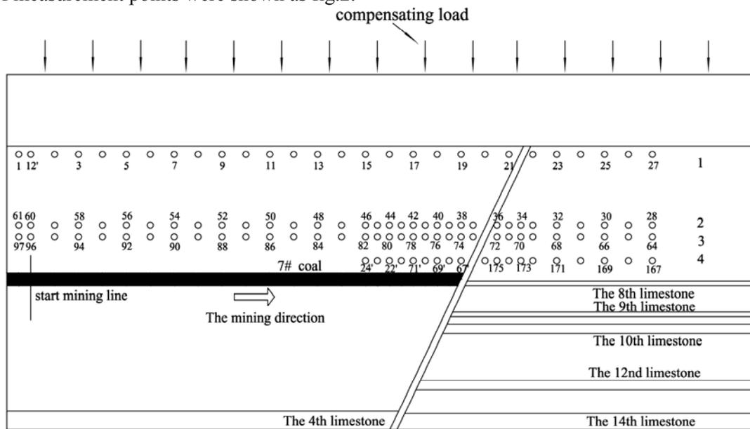
**Fig.2** Mining sequence and arrangement of measuring points of the simulated model
