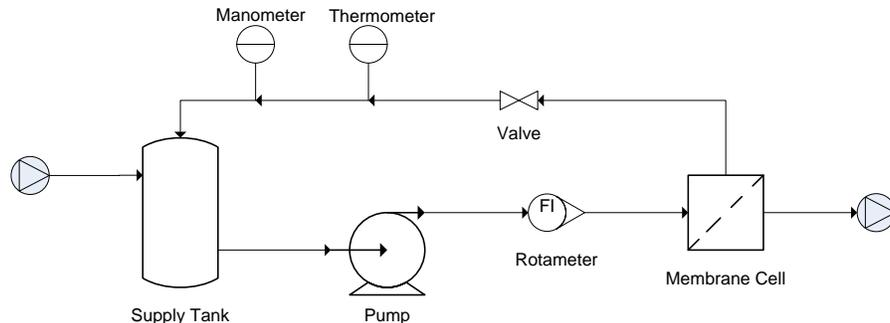
**Figure 1** Schematic of NF and RO unit
