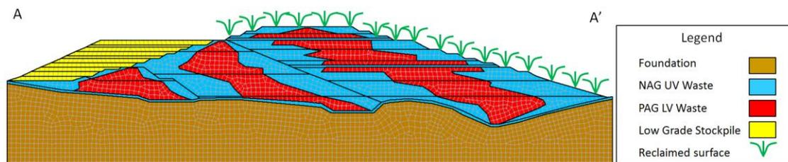
Figure 5 Cross section along axis of BRSF
