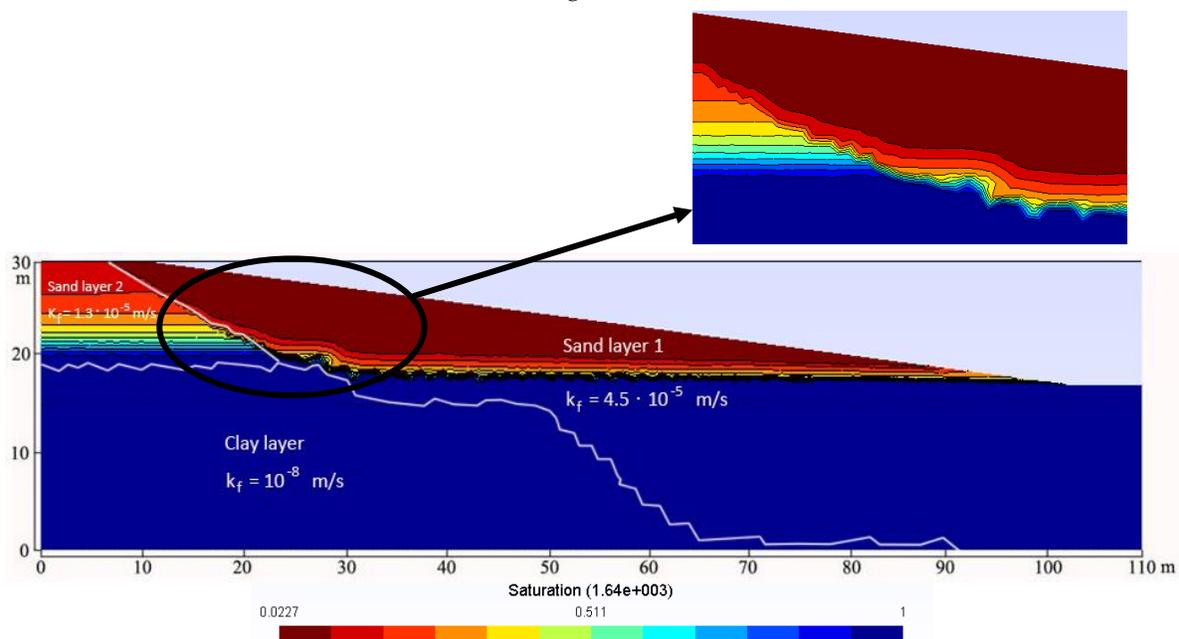
**Figure 5** Water saturation simulation without input of precipitation on June 30<sup>th</sup>, 2004 (the white lines are the borders of different soil layers with different hydraulic conductivity)
