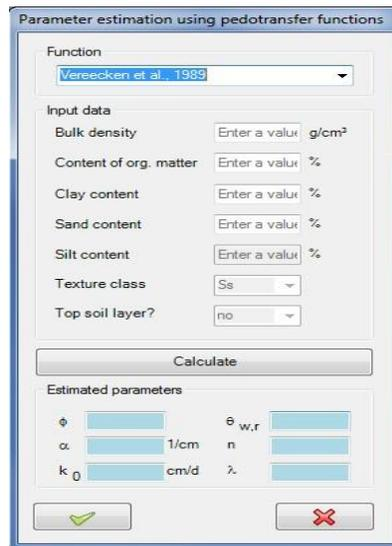
**Figure 3** Operation interface of parameter estimation using pedotransfer function in PCSiWaPro<sup>®</sup>
