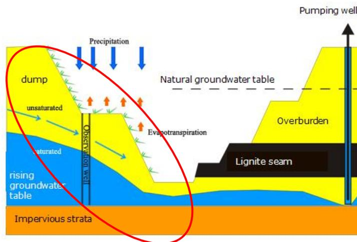
Figure 2 A simplified structure of the dump site
