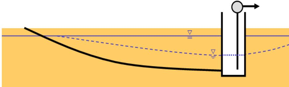
**Figure 4** Close-to-surface HDD filter well with collection shaft
