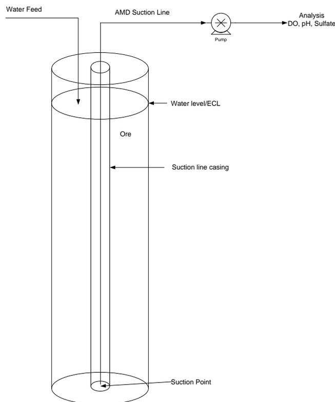
**Figure 3** Column reactor, showing feed ingress at the top and effluent removal via a casing in the centre of the column
