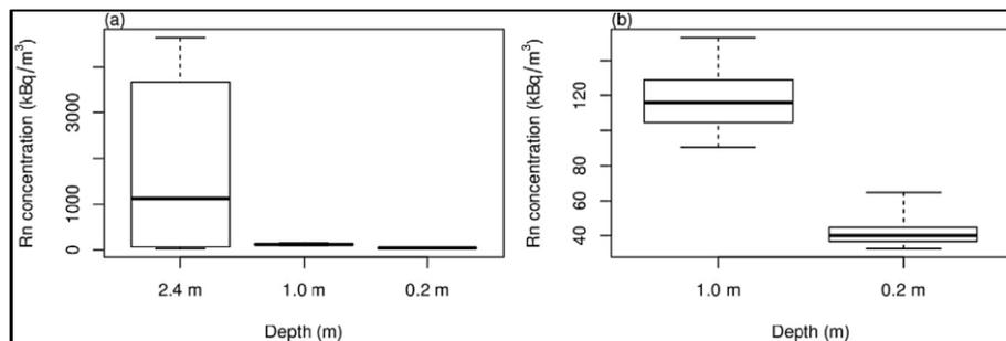
**Figure 4** Boxplots of the radon concentration values (left) measured at the 3 depths and (right) detailed view for the shallower measurements (Barbosa SM *et al.* 2015).
