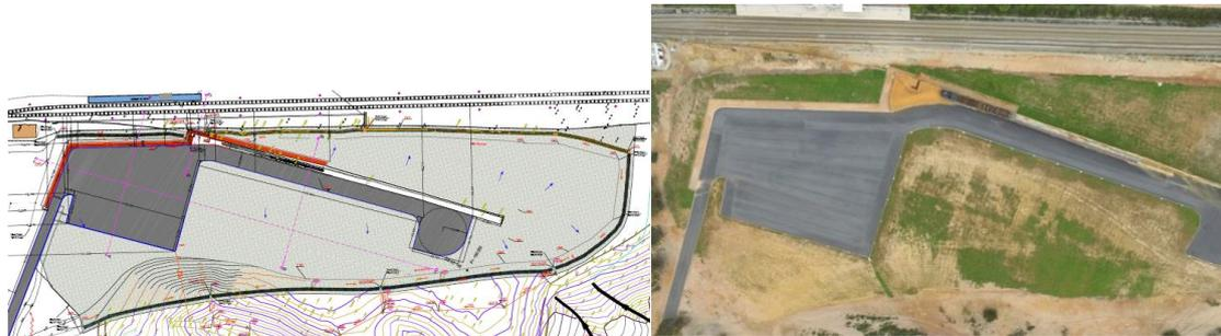
**Figure 6** HDPE and asphalt cover system in Lousal old mining area and photography after remediation works.
