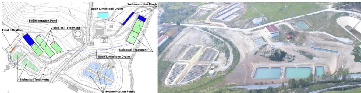
Figure 10 Cunha Baixa passive treatment process and photo.
