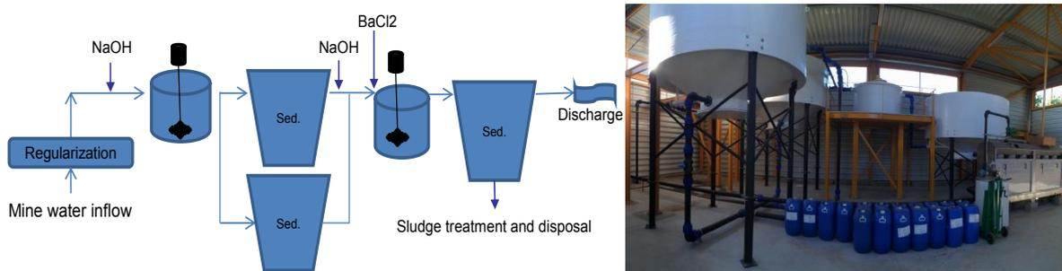
**Figure 9** Cunha Baixa active treatment process and photo.
