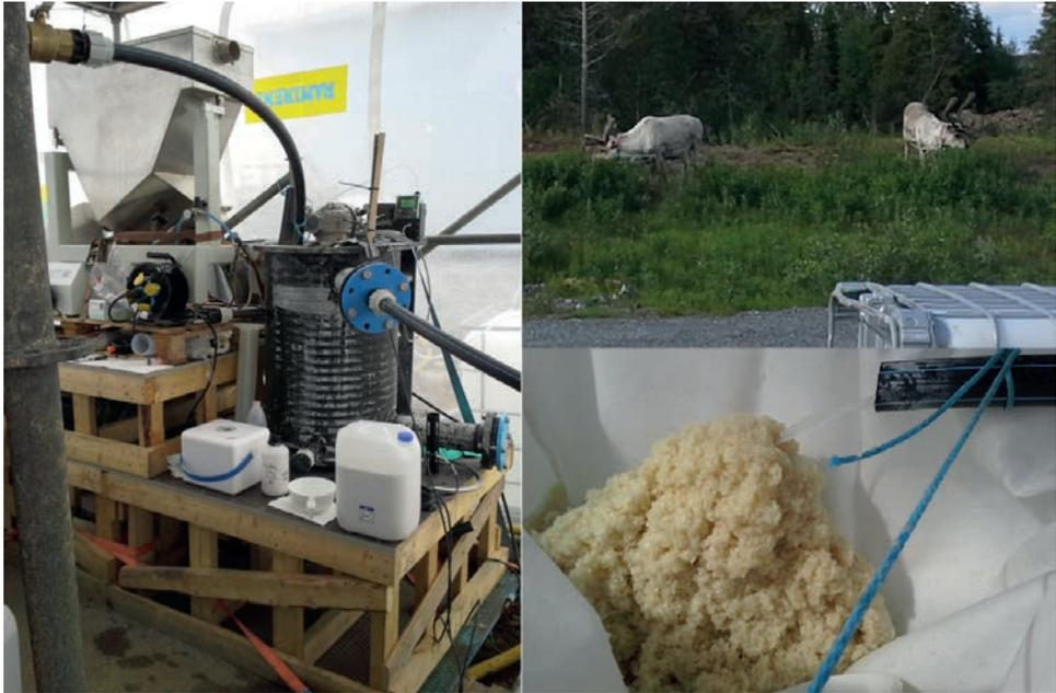
**Figure 3.** Pilot testing of biopolymer based sulfate removal system: part of used pilot equipment (left), pilot supervisors (top right) and sulfate containing biopolymer sludge (bottom right).
