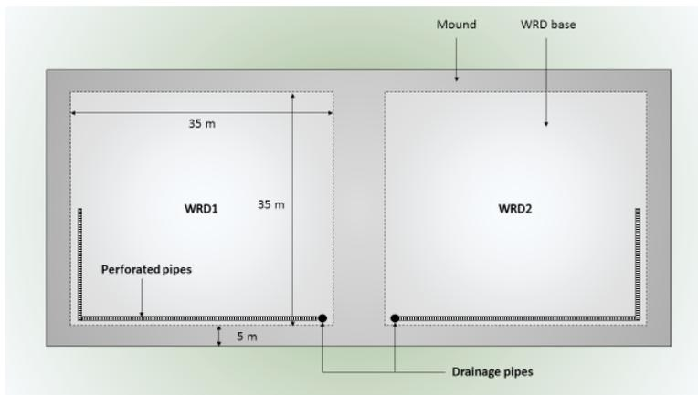
**Figure 1** Dimensions of the basal area of waste rock deposit with drainage. Light gray surface is the inner area, while the dark grey borders are the berms. WRD1 = south dump, WRD2 = north dump.
