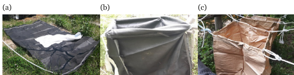
Figure 1 Materials for self-filtration: a: geotextile tube, b: geotextile bag, c: gunny bag.
