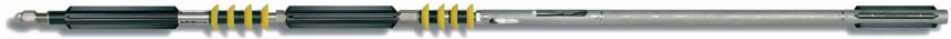
Figure 1 PFL tool with measurement section setup. Yellow disks are used to isolate measurement section from rest of the borehole.
