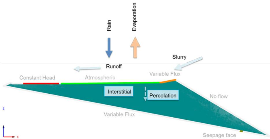
**Figure 1** Illustrated processes and boundary conditions of the 2D simulated tailings dam
