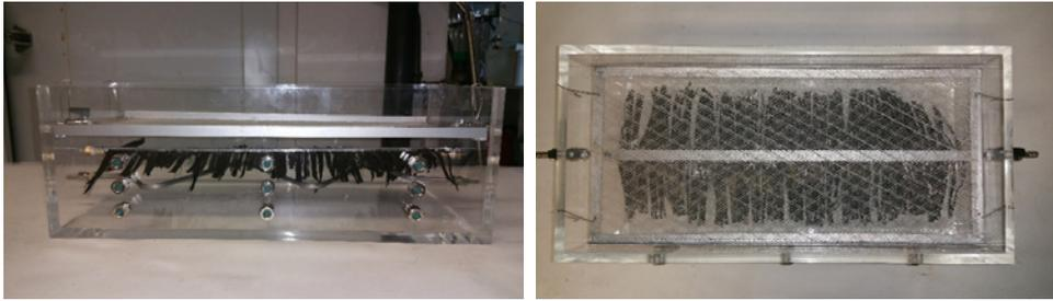
**Figure 1:** Images illustrating the LFCR design a) side view b) top view of the 8 L LFCR prior to inoculation fitted with strips of carbon microfibers, heat-exchange coil and harvesting mesh plate.
