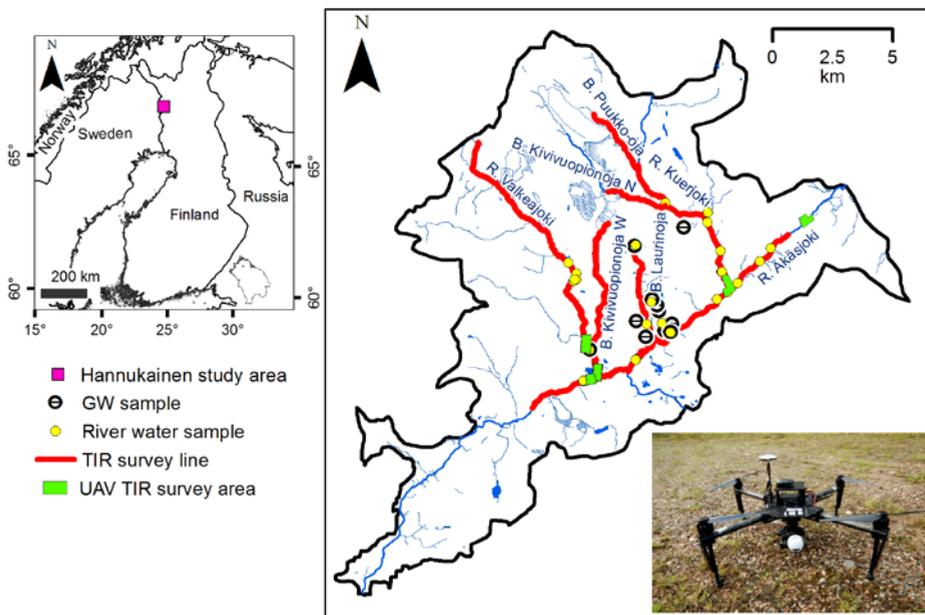
**Figure 1.** The coverage of helicopter-based TIR survey flight lines in 2012 and 2013, and UAV TIR survey areas, including the TMF 1A option and stable isotope water samples, as well as the used UAV platform (Matrice 100) with TIR and RGB cameras (Topographic Database © NLS 2016; Watershed Database © SYKE 2010).
