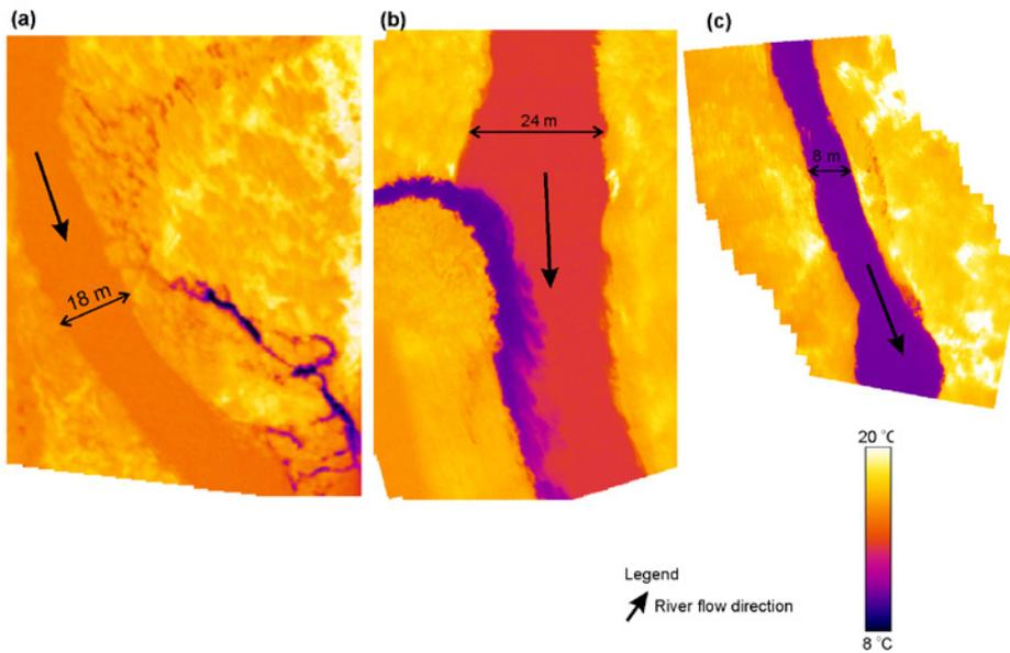
**Figure 3** Categories of discrete and diffuse thermal anomalies in thermal mosaic images; (a), seepage, (b) a cold tributary (R. Valkeajoki discharging into R. Äkäsjoki) and (c) diffuse discharge. The black arrows indicate river flow directions.
