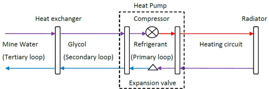
**Figure 1** Schematic diagram of heat pump system installed at Dawdon
