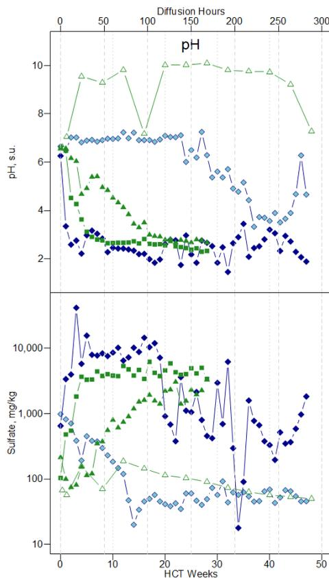
**Figure 2** Sulfate release and pH in kinetic tests of tailings
