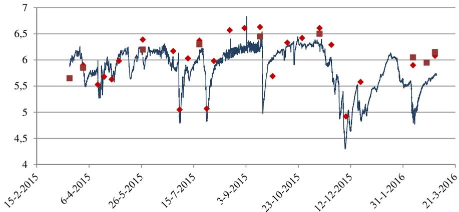
**Figure 3.** pH results of online measurement (solid line) and laboratory analysis of manual water samples (marked as rhombus and square representing different laboratories)
