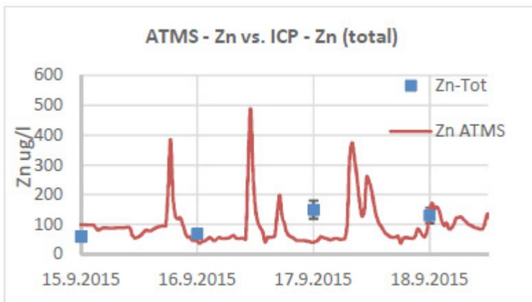
**Figure 2.** Comparison of online measurement data for Zn with online analyser and reference analysis results for total Zn concentration.
