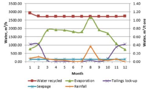
**Figure 6** Water in Thickener Tailings Management
