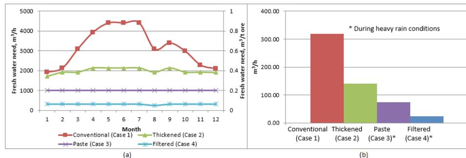
**Figure 4** Risk related to seepages from tailings management facilities at an arid region. Monthly fresh water make-up of the plant (a) and the estimated total seepage from the tailings facilities (b)
