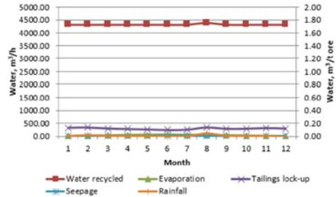
Figure 8 Water in Filtered Tailings Management
