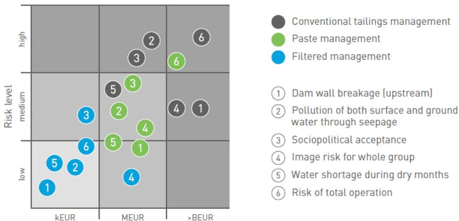
**Figure 2** Risk matrix for the assessment of operational risks associated with different tailings management processes
