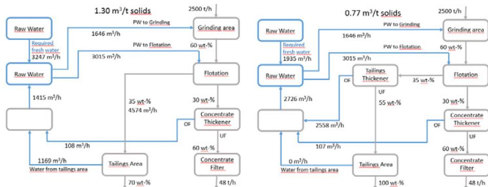
Figure 5 Simplified water balance calculations for conventional tailings (a, on the left) and for thickened tailings management (b, on the right)
