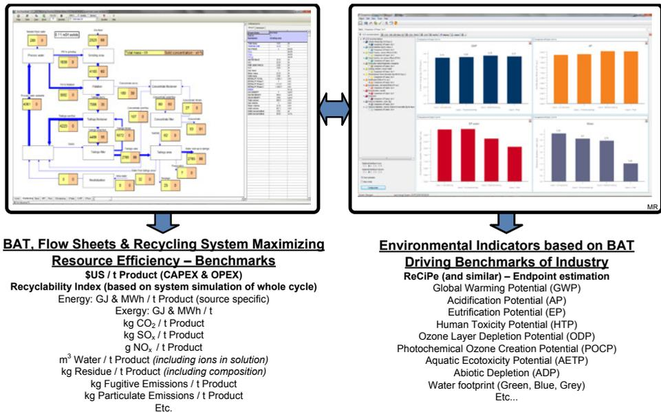
**Figure 1** Summary of the methodology: Left the HSC Simulation ([www.outotec.com](http://www.outotec.com)) of the water system for the four cases and right the environmental footprint calculation produced from the simulation results by life cycle assessment tool GaBi ([www.thinkstep.com](http://www.thinkstep.com)) (Reuter et al, 2015).
