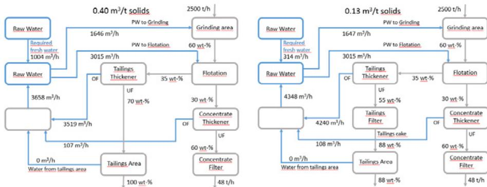
**Figure 6** Simplified water balance calculations for paste thickening (a, on the left) and for filtered tailings management (b, on the right)
