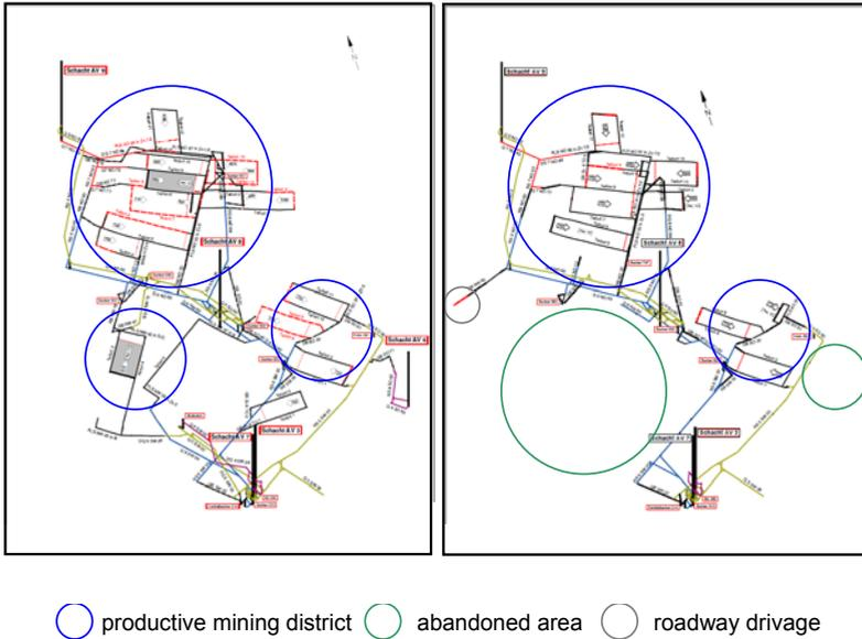
**Figure 4** Exemplary comparison of retreating areas in a mine
