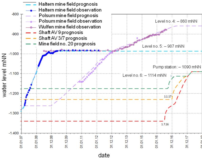
**Figure 6** Simulation of exemplary mine water levels and monitoring results (DMT)
