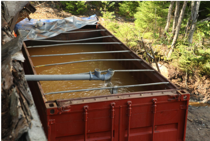
Figure 2 Picture of the Metsämonttu VFR at the end of the initial filling period (2016-08-08), before the installation of the aeration device.
