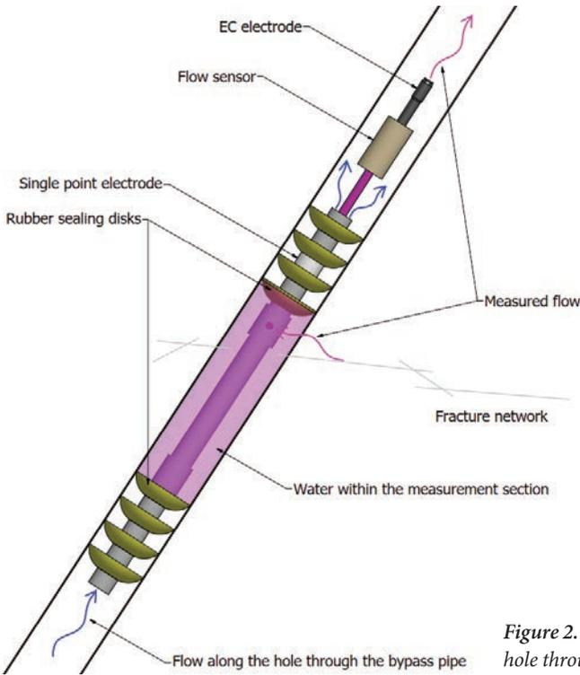
*Figure 2. Flow from the bedrock into a borehole through the flow sensor in a PFL probe.*
