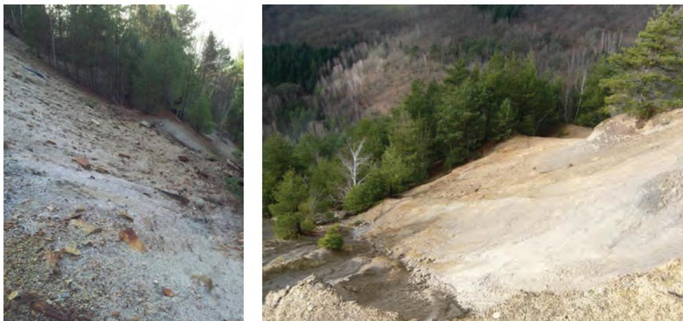
**Figure 4** As-bearing coarse gravity sorting residues in dumps (left) - eroded As-rich flotation residues in gravity dumps (right)
