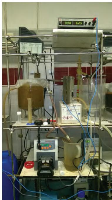
Figure 1 Set-up for a continuous electrocoagulation
