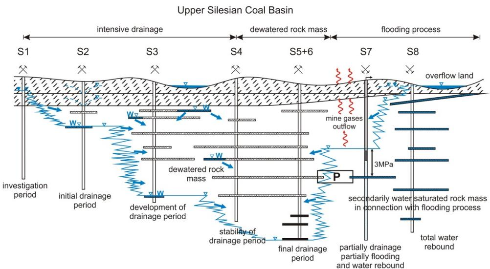
*Figure 1 Scheme of actual hydrodynamic situation of mining in the Upper Silesian Coal Basin and their possibility of influence on geomechanical and hydrogeological conditions and their changes*
