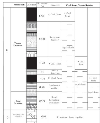
Fig 2. Hydrogeological column generalization of Yangjian Coalmine
