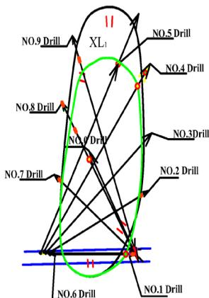
Fig 6. Design and layout of  $XL_1$  collapse column
