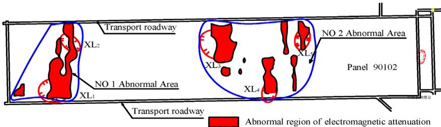
Fig3. Perspective of tomography in tunnel of panel 90102
