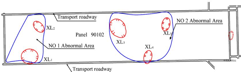
Fig4. Perspective of geophysical prospecting results in tunnel Panel 90102
