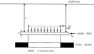
Figure 4. Theory of a Massive Bed Bridging over and Excavation.
