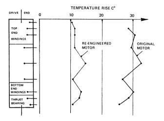
Figure 4 Submersible motor temperature profile
