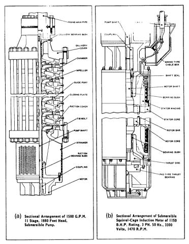
Figure 2 Typical submersible pumpset
