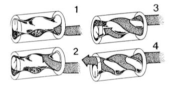
Figure 1 Stages for the screw-type pump
