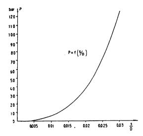
P = static pressure(bars), s = wall thickness (mm), D = casing diameter (mm)
