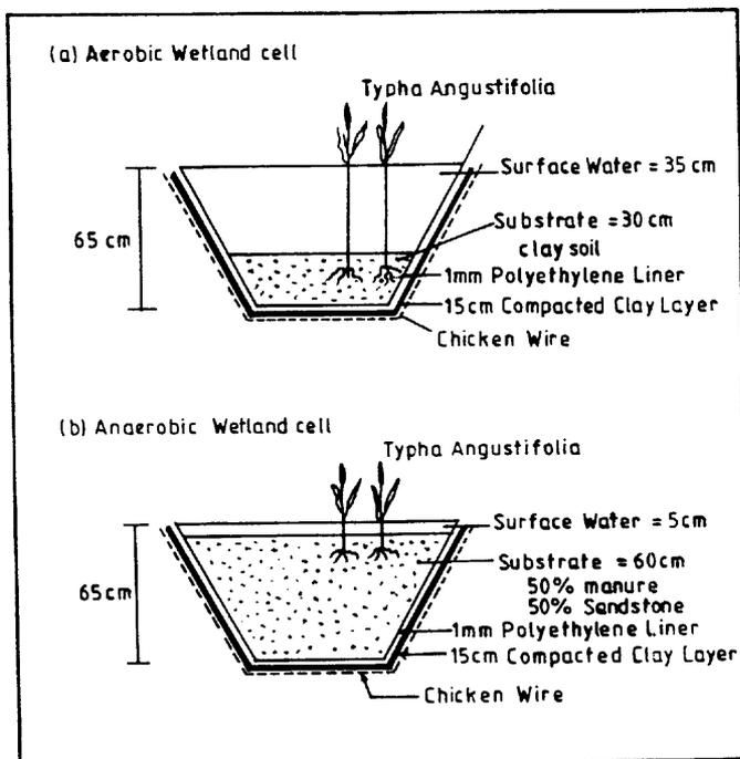
Figure 2 Typical design of aerobic and anaerobic wetland cells (Donahue, 1994)
