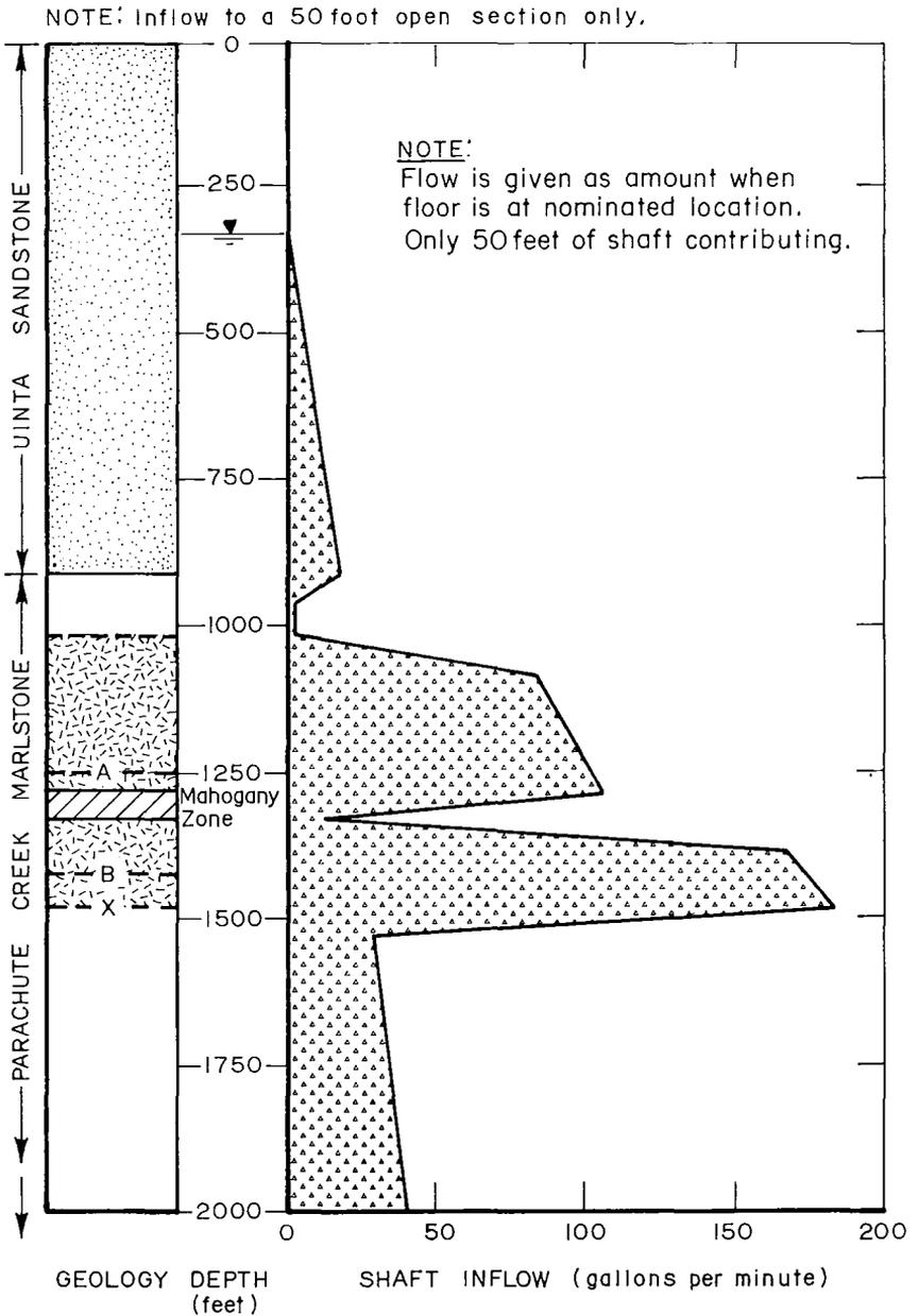
Figure 5 - Average Flow To Shaft Without Dewatering
