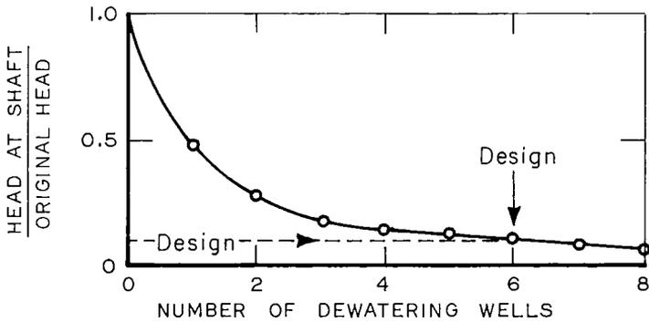
B) HEAD AT SHAFT IN LOWER AQUIFER VERSUS NUMBER OF DEWATERING WELLS.
