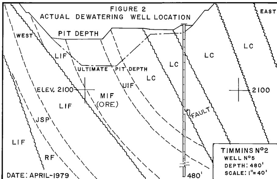
Actual Dewatering Well Location at Timmins 2 Mine. Figure No. 2.
