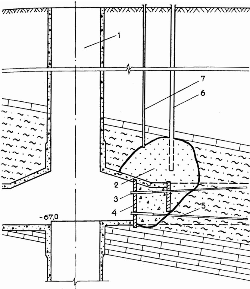
Fig.2. Diagram of consolidation in unstable aquiferous rock
