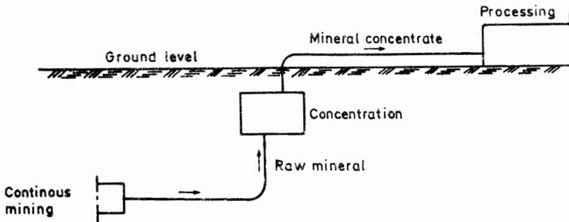
Figure 9. Continuous mining and long-distance pipeline transportation to processing plant.
