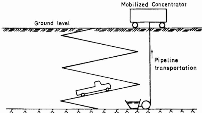
Figure 5. Hydraulic hoisting of ore in a small mine.
