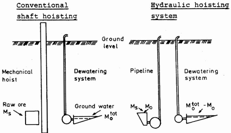
Figure 2. Flow of raw ore and mine water in a conventional shaft system and in a hydraulic hoisting system.
