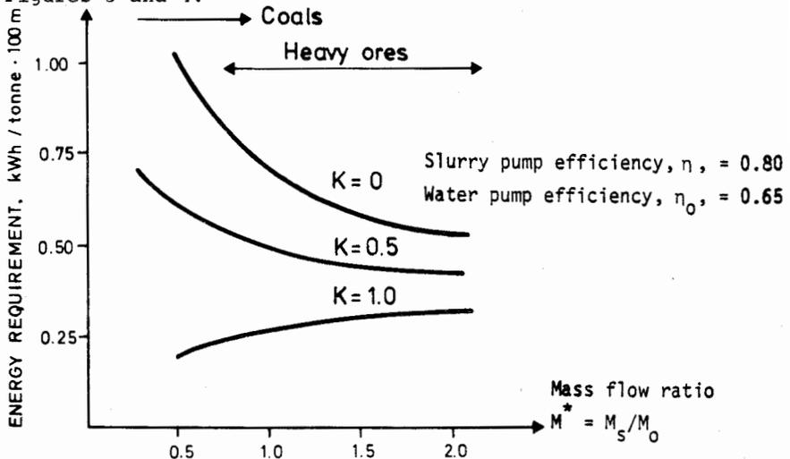
Figure 3. Net energy requirement in a hydraulic hoisting system based on high-efficiency slurry pumps.  $K$  is the amount of water needed which is available underground.
