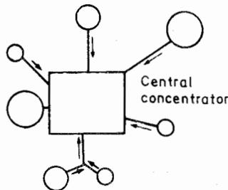
Figure 7. Hydraulic hoisting and haulage to a central concentrator from a group of underground mines.
