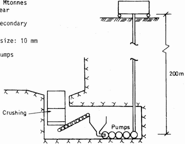
Figure 6. Layout of a hydraulic hoisting system in a small mine.
