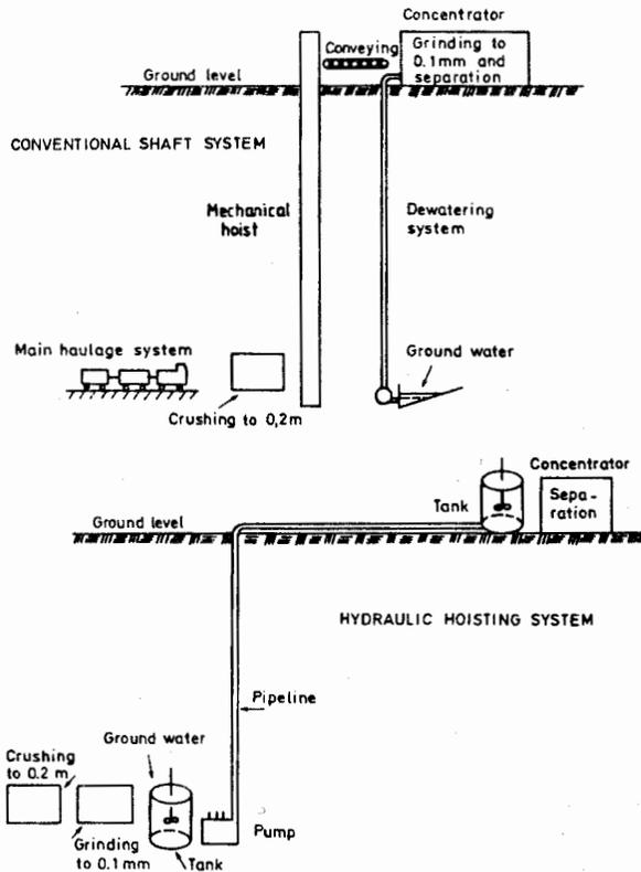
Figure 1. Schematic layout of a hydraulic hoisting system compared with a conventional shaft hoisting system in an underground mine.
