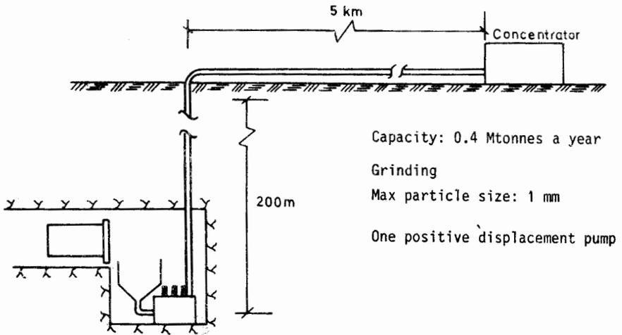
Figure 8. Slurry transportation to a central concentrator.
