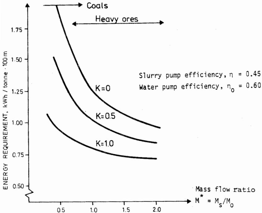
Figure 4. Exemplification of the net energy requirement in a hydraulic hoisting system based on centrifugal pumps.
