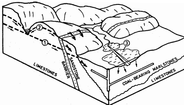
**Fig.2 Schematic block-diagram of the Bogovina mine flood.**
