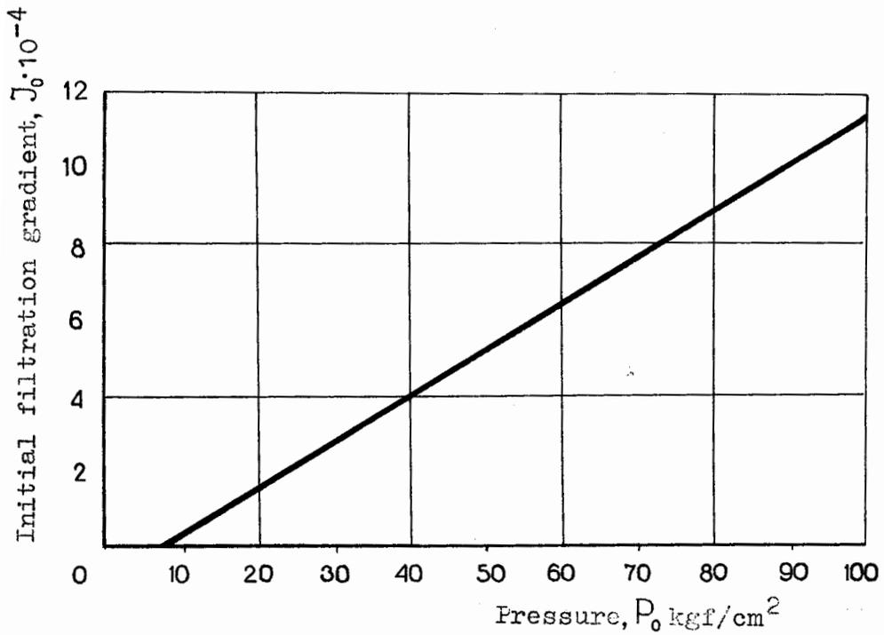
Fig. 2 Initial filtration gradient and grout cover formation pressure relationship
