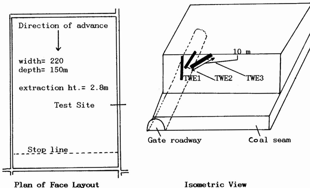
Figure 5. Test Layout on Retreating Face
