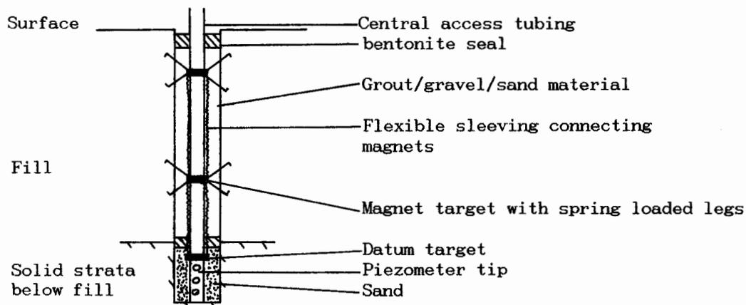
Figure 6. The Magnetic Extensometer/Piezometer Instrument
