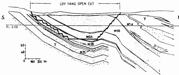
Figure 2: Geological Cross-Section of Loy Yang Open Cut
