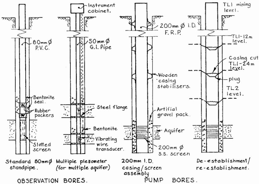
Figure 4: Typical Observation and Pump Bore Designs
