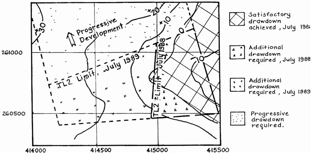
Figure 3: Loy Yang Open Cut, Block 1. Aquifer Pressure Target Plot for M2B Aquifer and TL2 Mine Grading
