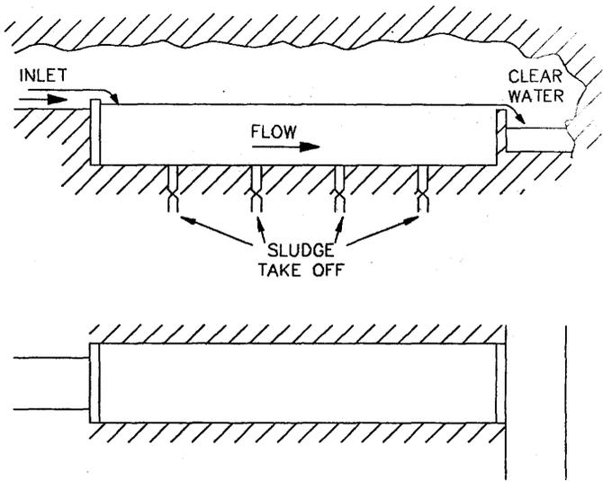
FIG. 1 RECTANGULAR HORIZONTAL FLOW SETTLER
