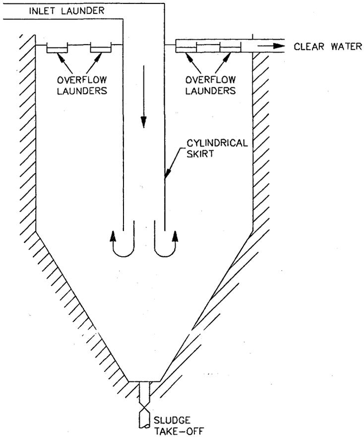
FIG. 3 MODIFIED VERTICAL FLOW CONICAL SETTLER
