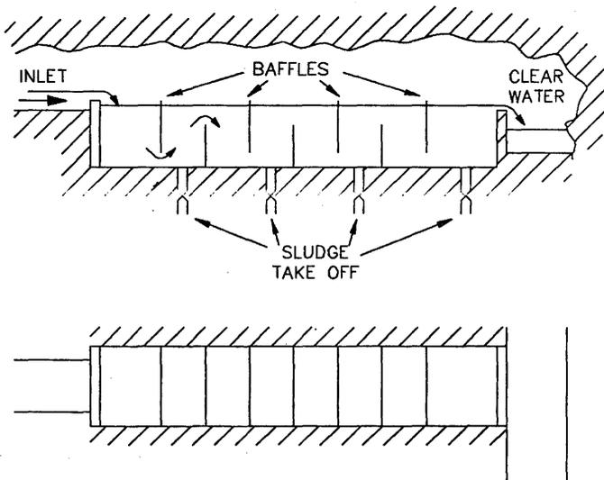
FIG. 1a MODIFIED RECTANGULAR HORIZONTAL FLOW SETTLER
