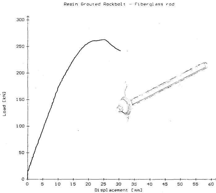
Fig. 13 Resin grouted rockbolt - fibreglass rod, tensile loading across a joint.
