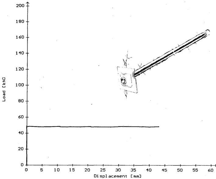
Fig. 14 Friction anchored rockbolt - Split Set, type SS 39, tensile loading across a joint.
