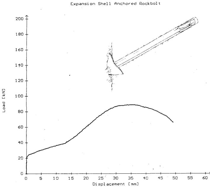
Fig. 10 Expansion shell anchored rockbolt, tensile loading across a joint.
