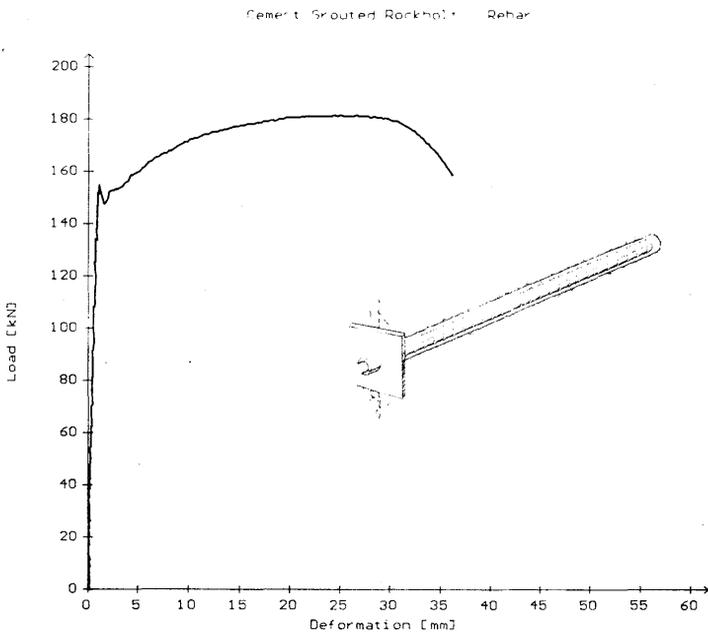
Fig. 11 Cement grouted rockbolt - rebar, tensile loading across a joint.
