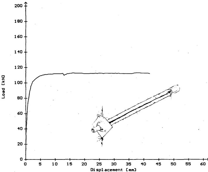
Fig. 15 Friction anchored rockbolt - Swellex, type EXL, tensile loading across a joint.
