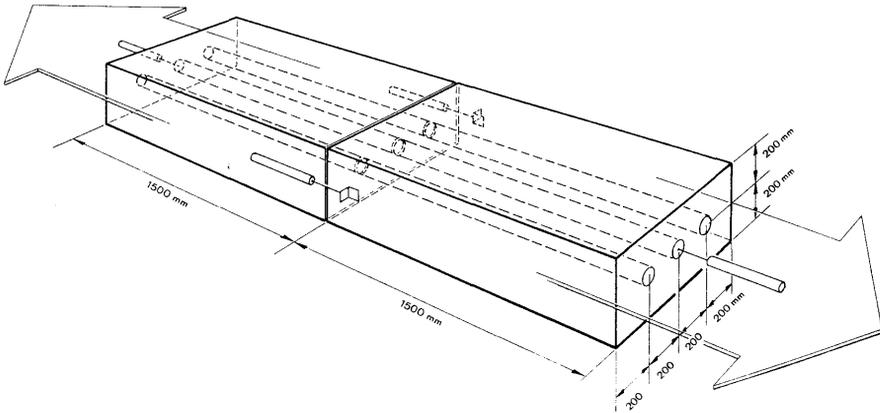
Fig. 8 Schematic illustration of the test arrangement for rockbolt tensile loading across a joint.
