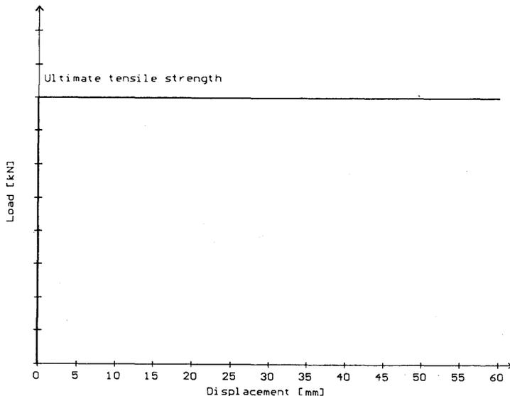
Fig. 1 The ideal load-displacement characteristics of an installed rockbolt, independent on ground conditions.
