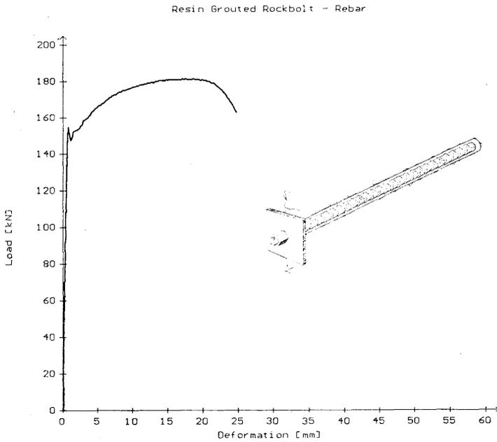
Fig. 12 Resin grouted rockbolt - rebar, tensile loading across a joint.
