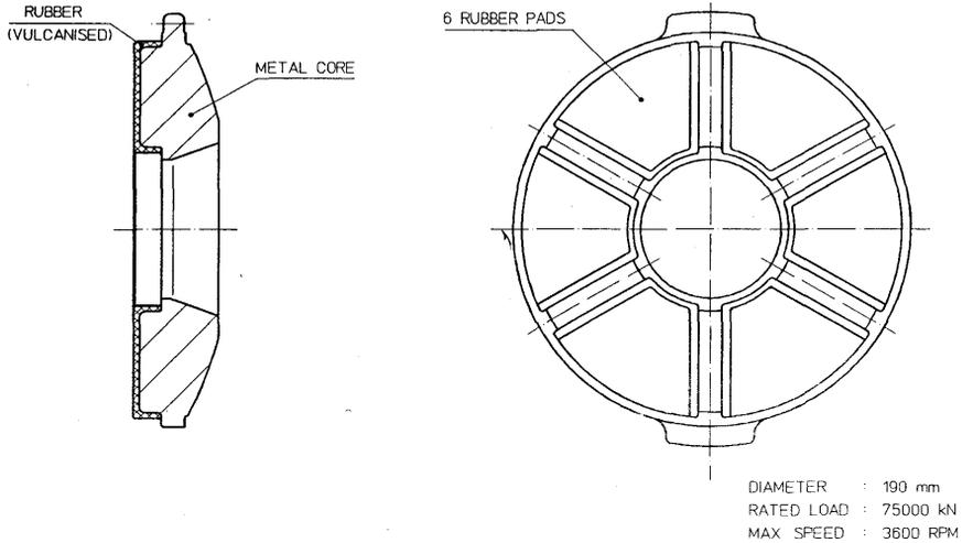
FIG. 5: FIXED PADS AXIAL THRUST BEARING
