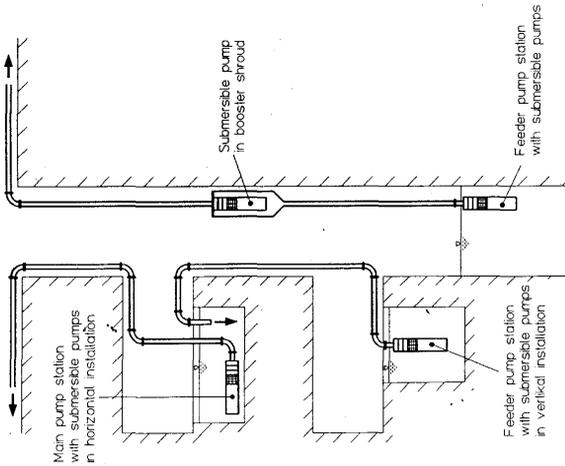
FIG. 1: DIFFERENT SUBMERSIBLE PUMPS INSTALLATIONS IN MINES
