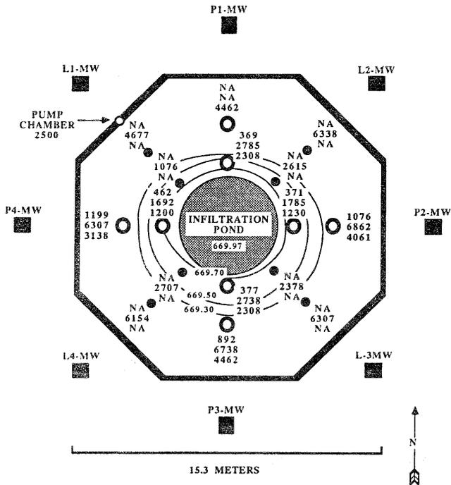
Figure 5. Spatial distribution of break through times (minutes) in the sandy-silt (top value), gray clayey-silt (middle value), and the gravel (bottom value). Steady-state potentiometric surface in the sand unit during CHST-2. Units of the contours are meters AMSL.
