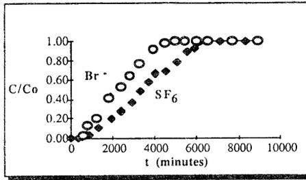
Figure 4. Break-through curves of  $\text{Br}^-$  (empty polygons) and  $\text{SF}_6$  (filled polygons) as observed at the pumped drain tile. Concentrations of each tracer measured ( $C$ ) are relative to the steady-state concentration in the pond ( $C_0$ ). See Figure 2 for the location of the pumping well.
