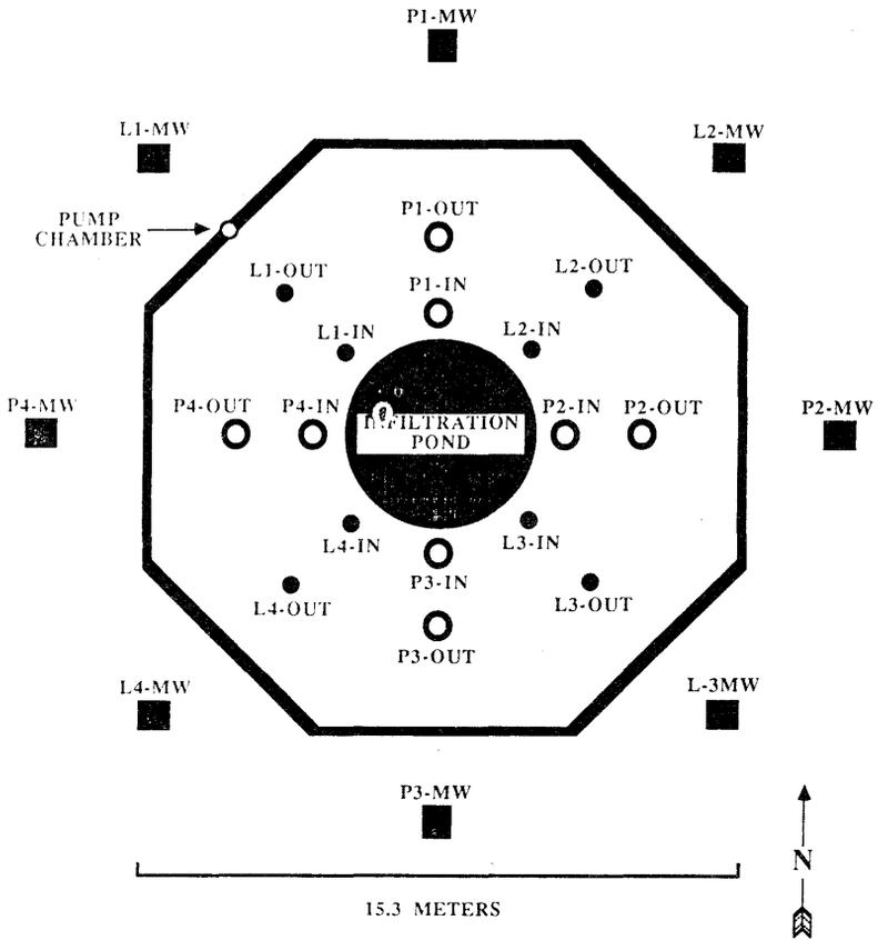
Figure 2. Plan view of the in-situ leach cell showing the locations of the drain tile (black octagon), excursion ground water monitoring wells (black squares), lysimeters (black filled circles), and piezometer nests. Nests consist of piezometers completed in the aquifer, gray clayey-silt, and sandy-silt units.
