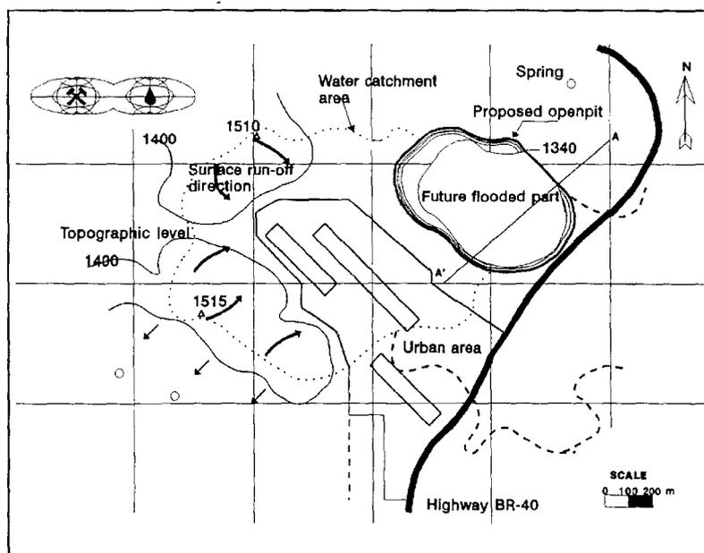
Figure 6. Schematic drawing of Capao Xavier Mine surface hydrological behaviour (FRASA, 1995).
