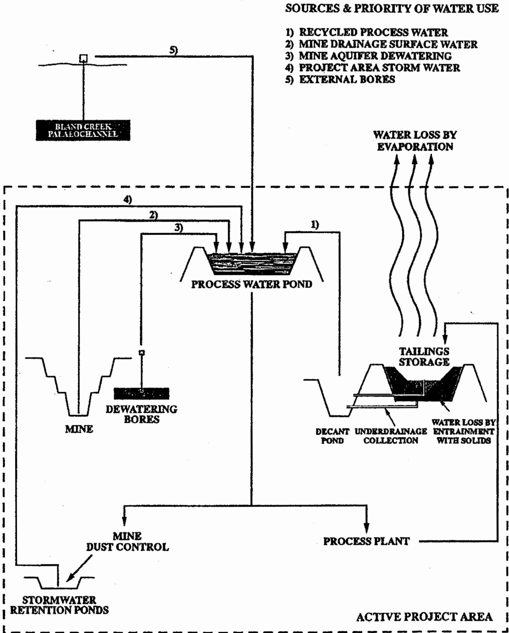
Figure 3: Mine water management flowsheet (after NSR, 1996)
