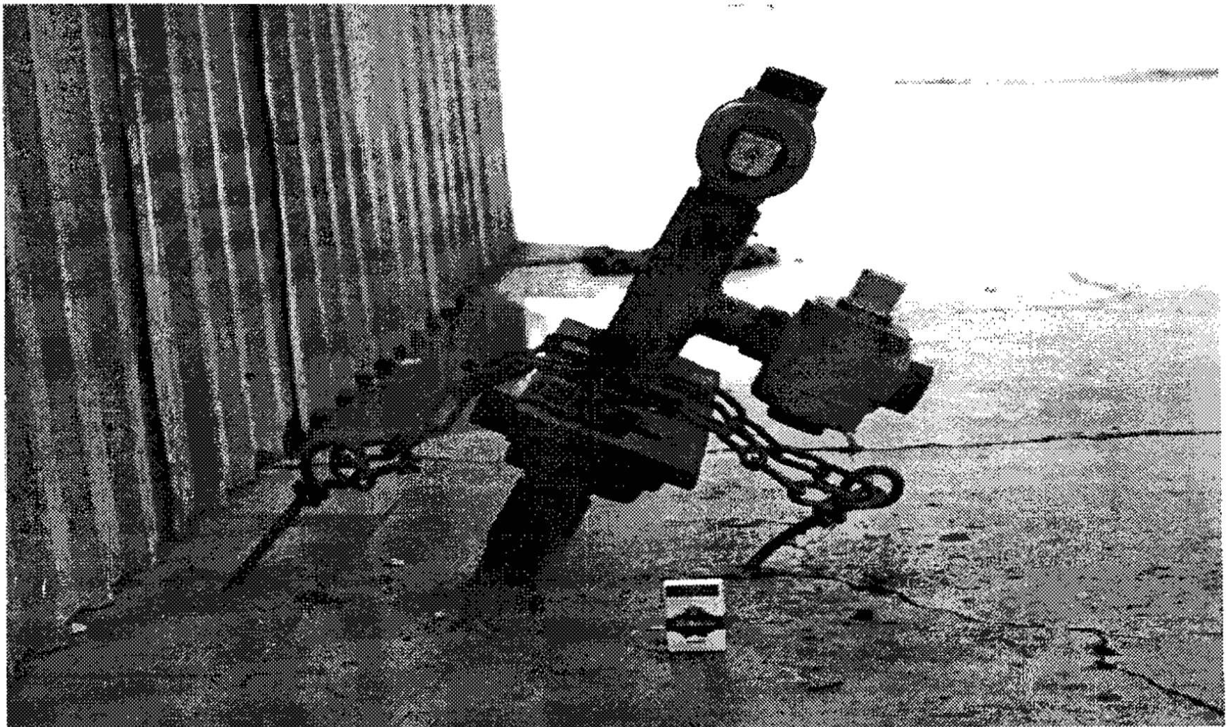
**Photo 2 : High Pressure Safety Valves. Side view.**
