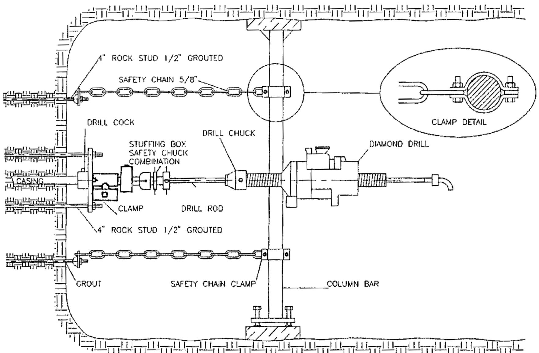
Drawing 1: Schematic presentation showing High Pressure Safety Valves configuration for High Pressure Drilling
