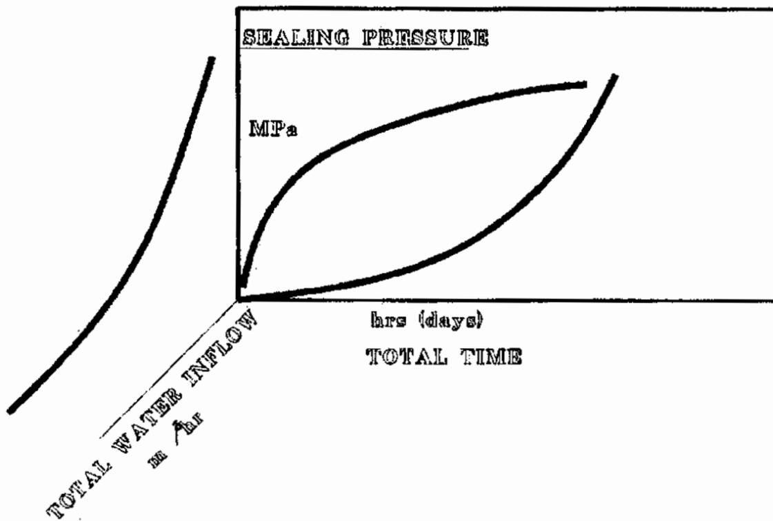
FIGURE - 5 : Total water inflow into mine as a function of sealing pressure typically used on mine.
