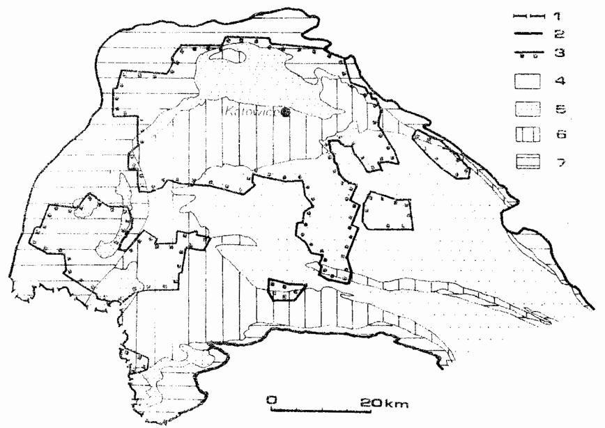
Fig. 1. Permian, Mesozoic and Cainozoic subcrop map of the Upper Silesian Coal Basin (USCB), with outlined of coal mine fields
