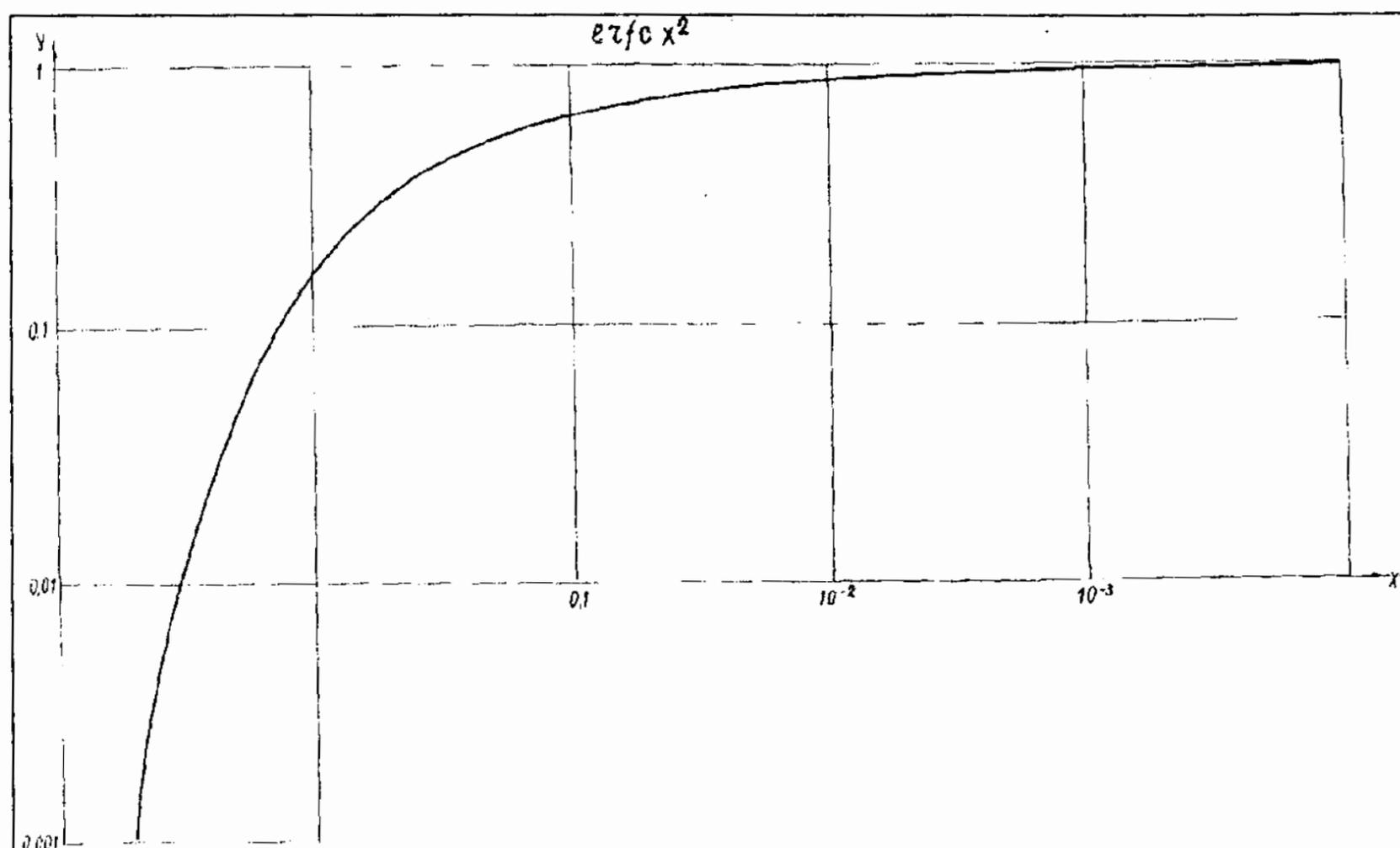
Fig.3. Type curve  $y = \text{erfc}(x^2)$ .
