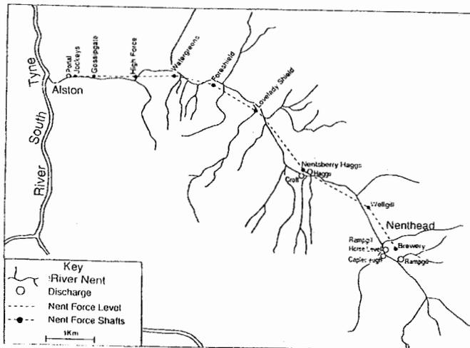
Figure 3: Map of the Nent Valley, Cumbria, UK, showing the surface trace of the Nent Force Level below the valley axis, the locations of air-shafts and access shafts along the Nent Force Level (black circles) and the positions of major adit portal other discharges (open circles) from perched groundwater systems in mine-workings lying above the level of the Nent Force adit.
