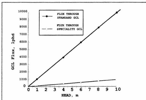
Figure 1. GCL flux as a function of head pressure. Flux testing was performed in a flexible wall permeameter under a constant confining stress of 35 Kpa (CETCO, 1996).
