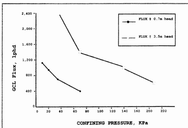
Figure 2. GCL flux as a function of confining pressure. Flux testing was performed in a flexible wall permeameter under head pressure of 0.7 m and 3.5 m (CETCO, 1996).
