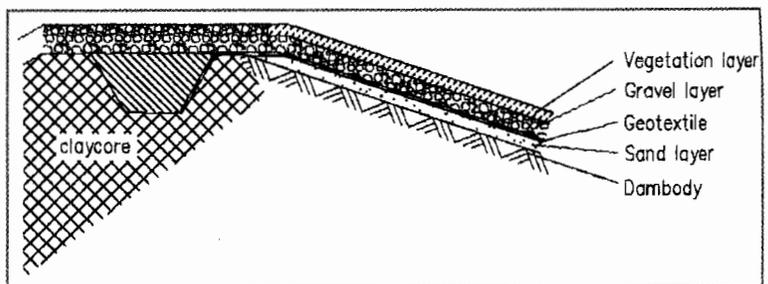
Figure 3. Geotextile on the downstream face of a slope as surface protection and protection of the top in case of an overflow.
