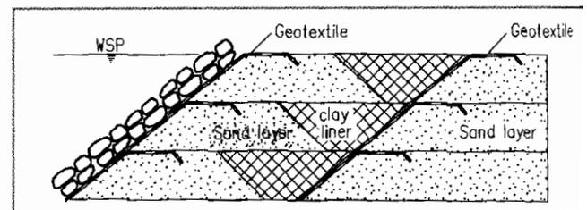
Figure 8. Installation of geotextiles as filter in the dam (hydraulic fill dams).
