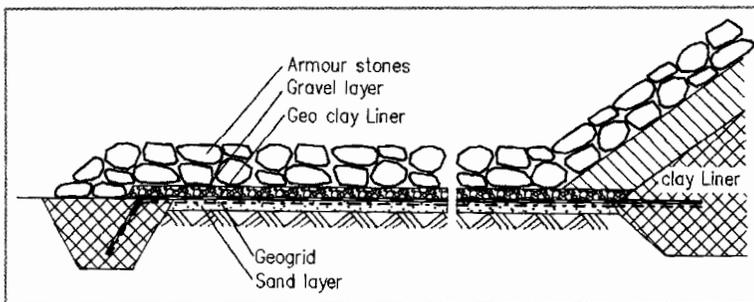
Figure 6. Elongation of the seepage way with geosynthetic liners for avoiding of piping.
