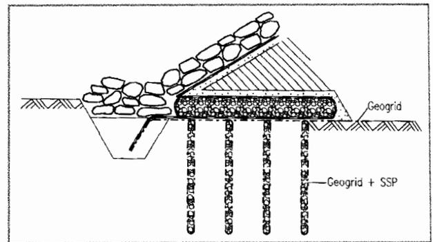
Figure 7. Shows the installation of a horizontal filter with vertical drainage and a geogrid with high tensile strength.
