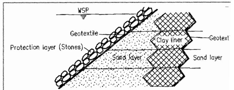
Figure 9. Installation of filtermats behind the core (hydraulic fill dam).
