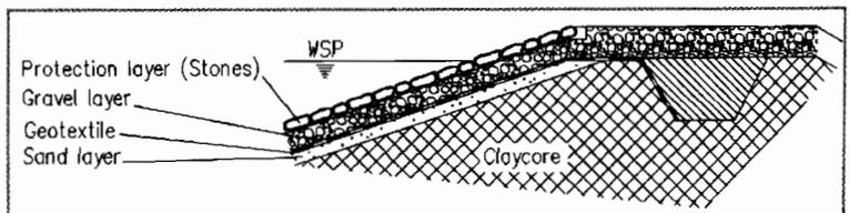
Figure 4. Geotextile on the upstream face as separation layer and filter.
