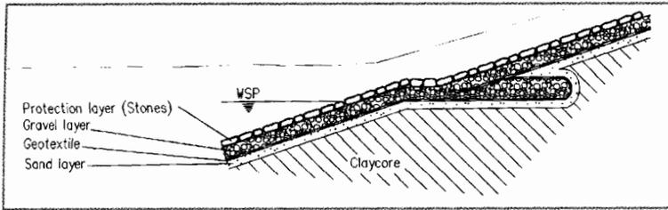
Figure 5. Surface filter with geotextile sheathing for increasing the safety of the slope in case of fast draw down or unsuitable dam material without sliding resistance.
