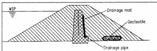
Figure 10. Expansion drain on the downstream face of the core.
