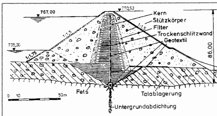
Figure 12. Frauenau-dam, cross section of the dam and details of the control passage.
